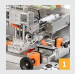
As well as a thermal transfer printer for variable data – typically the batch number and expiry date – the pharma equipment includes the integration of various camera systems to verify printing and codes.
