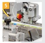
For labeling frequently changing products with different dimensions, format parts with quick-change unit can be supplied as an option. This allows easy format changes at any time without long changeover times.
