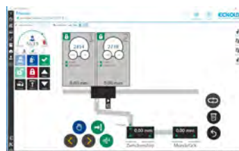
Connected rivet feeding stations are also monitored.
