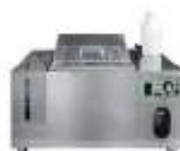
▲ Salt Spray Test
