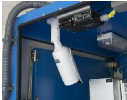
Camera for observation of interior machine
