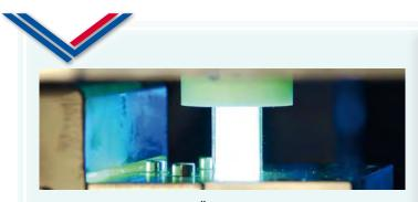
Another innovation of HÜBERS is the procedure for the **processing of UV-silicones**. In this case the material is exposed to UV light and thereby activated before the injection into the mold. After activation, the vulcanization of these special silicones is greatly accelerated. For certain components the cycle times in the form could be reduced by up to 65%.
