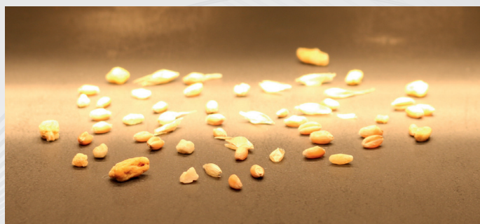
figure 1: Sample on the scanning table (mix of corn, stones, empty shells and wood)
