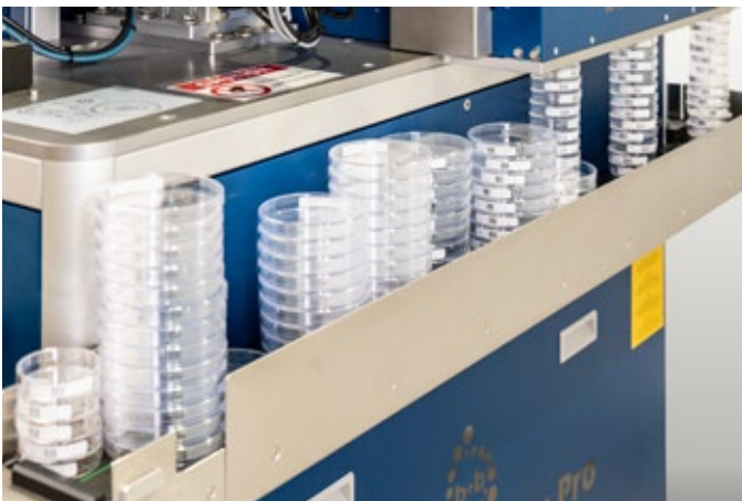
Figure 3: The circulating discharge conveyor transports the stacked Petri dishes to the front of the system
