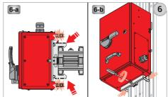
6-Push the box into the Busbar housing a "click" sound will be heard from the locking parts of the box ensure that it interlocks with the box and the housing thereafter tighten the screw.
