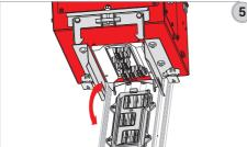
5-Check the alignment of the contacts. Push the box towards the Busbar.
