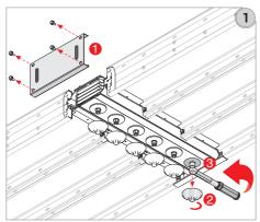
1-Remove the locking pieces. Remove the joint side cover plate and keep the plate and the screws for future use
