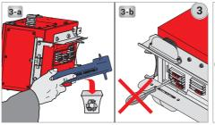
switch to zero position. As seen on figure 3-b, do not interference with the jawed contacts. Do not deform box upwards as shown in figure 4-b. them.
