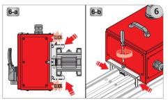
**6**-Push the box towards the Busbar housing a "click" sound will be heard from the locking parts in the box, ensure the interlock between the box and the housing and thereafter tighten the screw.
