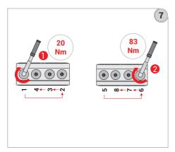
7- If there are more than one bolt for the same phase, bolts shall be tightened by hand to approximately 20-30Nm as per above illustration, then 83Nm shall be applied for the final torque using the same sequence.
