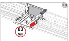
10- Adjust the torgue wrench to 83 Nm (60 lbft) and tighten the joint nut.
