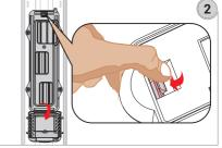
2-Open and push the cover back. The "plug-in" tap off point cover should be opened to a position which will not block the way for installation of the box. Do not remove the cover plate.
