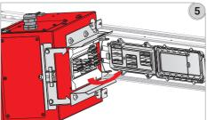
**5**-Check the alignment of the contacts. Push the box towards the Busbar.
