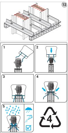
14- Ensure the selected degree of protection (IP rating) of the system is suitable for the working environment.
