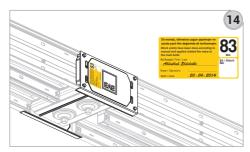
**14-** Please complete the label attached to the joint cover to verify that you are performing torque settings according to the specifications.
