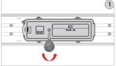
1-Remove the fixing screw of the "plug-in" tap off point cover using a star screwdriver.
