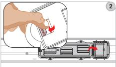
**2**-Open and push the cover back, the "plug-in" tap off point cover should be opened to a position which will not block the way for installation of the box. Do not remove the cover plate
