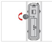
1-Remove the fixing screw of the "plug-in" tap off point cover using a star screw driver.
