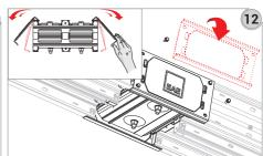
12- Remove the joint covers and reverse mount them with the gaskets facing inwards.
