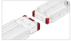
1- Align the two Busbars so that the sections with and without block joints are opposed.
