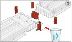
2- Remove the protective side covers on the no block joints.
