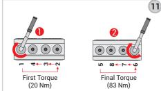
11- If there is more than one bolt per phase, the bolts should be tightened by hand to approximately 20-30 Nm as per the sequence shown above. Then finally torque to 83Nm using the same sequence.
