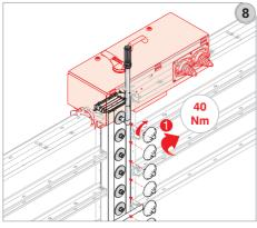
**8-** Then tighten the locking piece to 40Nm to complete installation(1).
