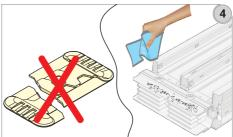
are not cracked, broken or damaged in anyway. Wipe the dust off conductor surfaces with a cloth, so that no serious damage can be caused.
