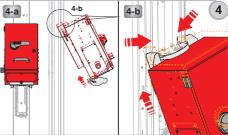
3-Throw the contact protection cover to the recycling 4-Place the KXP Plug-in tap off box into the waste bin. Make sure that you have brought the holes on the Busbar at an angle. Push the tap off
