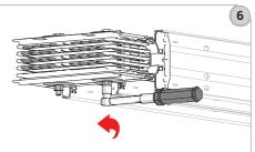
5- Align the block joint to the opposite busbar's 6- Loosen the nut at the connection point. end.
