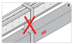
**8-** Do not use busbar system as a supporting structure for other systems.
