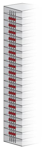
In multi-path Busbars in high-rise vertical shaft applications; Due to floor heights, floor thickness and product tolerances, the window or additional point alignments on the upper floors may not be the identical. In order for the Tap off boxes to be aligned and the joint point not to coincide with the floor transitions, the assembly should be continued by creating measurements on each floor.
