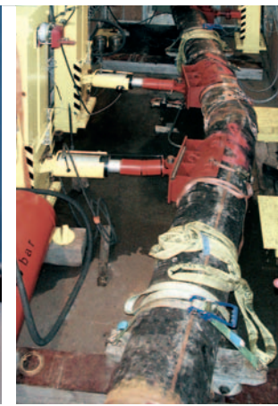
From left to right Residual stress measurements by hole drilling method Tensile test on pipe material Laser-scan test on pipe joint Bent pipe segment with special joint under internal cyclic pressure in burst test pit
