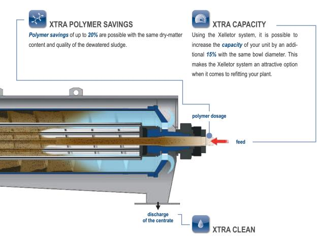
In sludge dewatering, the **separation efficiency** of our centrifuges is in general greater than **99%**, which reduces back-contamination in the centrate and thus saves additional costs.
