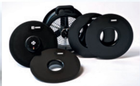
BlowerDoor flow rings until 1991 (left), BlowerDoor flow rings since 1992 (middle), set of flow rings BlowerDoor MiniFan since 2014 (right)
