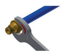
**Step 5**Tighten forcing nut firmly.
