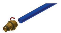
**Step 3**Unscrew the forcing nut except of two turns.
