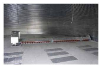
Silos Spain sweep augers adapt to our silo diameters and can be complemented with accessories that enhance emptying by eliminating all existing residue between the sweeping machine and the ground. Complies with the ATEX standard for work inside a silo.
