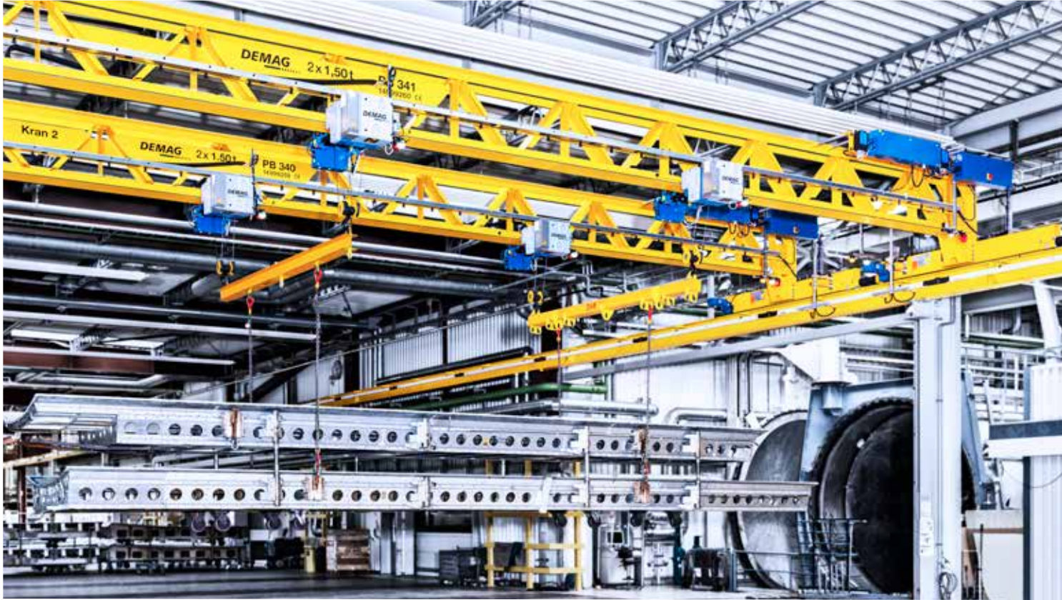
Smart tandem with up to four synchronised hoists and two cranes.
