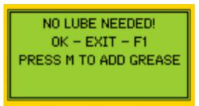
LUBRICATION NOT NEEDED message is assigned automatically and marked as an automatic status/action message;
