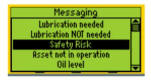
By pressing ENTER, you acknowledge that you are at the RIGHT POSITION at the RIGHT INTERVAL, using the RIGHT LUBRICANT and the RIGHT GREASE GUN. You are also informed if there is an alarm assigned to this position (or not) and if yes, what is the threshold. In case you have multiple alarms, LUBExpert will display lowest (tightest) one that will trigger your decision to apply grease.
