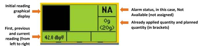
(In cases when alarm is assigned and triggered, alarm level will be displayed on screen)
