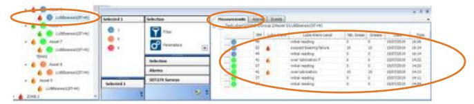
This view gives many different information sets. You can customize your view in the Parameters Menu. In the view displayed in the above screenshot, we see Alarm Level, RMS value for each measurement, Lube Alarm Status, Lube Alarm Level Specified, Number of Shots Added, Quantity of Added Grease in Grams (oz), Date and Time.
