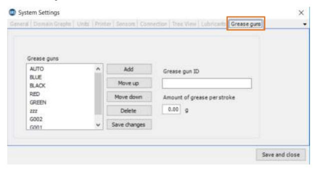
UAS3 and LUBExpert want to ensure you always use the right grease and the right amount. To accomplish this, you need a tool to manage your grease guns. To manage multiple grease guns in
