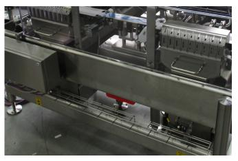
The combined device offers a total of four boxes for the rejected goods.
