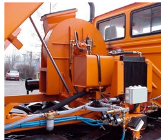
Gas-tight radial fan in two-stage design for transporting hydrogen
