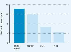
Comparison on a 4.8 mm screw with fillister countersunk head at contact pressure of 23 N.
