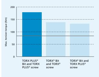
Typical tightening torque for a 7/16" screw quality 10.9. Test results from investigations made on TORX PLUS® 50IP and TORX® t50.
