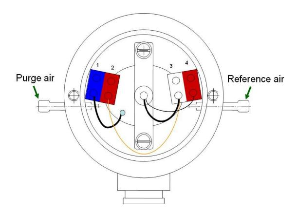
Important notice! To avoid plugging use a filter between the pump and the probe! To avoid damages only use clean and dry air as reference and purge air.
