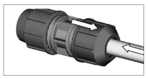
**Step 3** Insert the pipe up to the stop.
