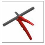
**Step 1**Cut the pipe at a right angle at the previously affixed marking.
