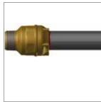
**Step 4**Insert the pipe up to the marking.
