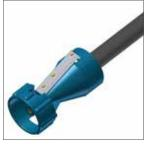
Step 2 Chamfer the pipe up to the inner diameter (e.g. with chamfering tool model 8880, item 124527).
