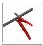
**Step 1**Cut the pipe at a right angle at the previously affixed marking.
