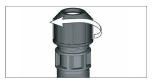
**Step 5**Put on the nut (1) and fasten it with one turn so that the pipe can still be pushed into the coupling.
