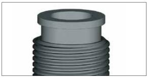
**Step 3**Put the sliding ring (3) with its flat side up on top of the seal.
