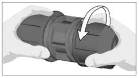
**Step 2**Loosen the nut without separating it from the housing.
