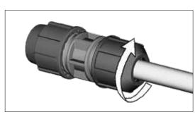
**Step 4**Tighten the nut firmly by hand and additionally by a tool.
