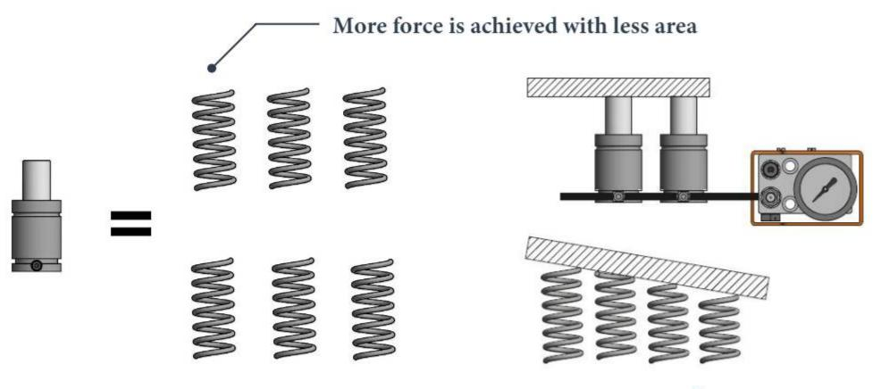
Force is balanced in serial connection systems created with gas springs. The pressure value can always be seen on the system.
