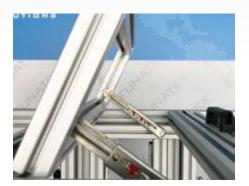
T-STEP is a user friendly, easy to use telescopic positioning stay. TGS offers this stays in three versions (5 step, 6 step, 10 step) which presents to operate up to 135 KG applications. In order to open, extend the arm until it locks into the desired position. To close, fully extend T-STEP before returning it to the closed position.
