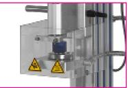
sealing head heating block with heat protection shield
