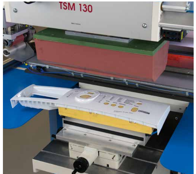
TSM 130 universal transverse doctor kit Jig with washing machine panel
