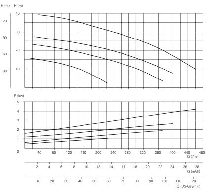
Characteristic lines measured with water, 20° C and 2900 Rpm (50 Hz.) chemical resistant pumps
