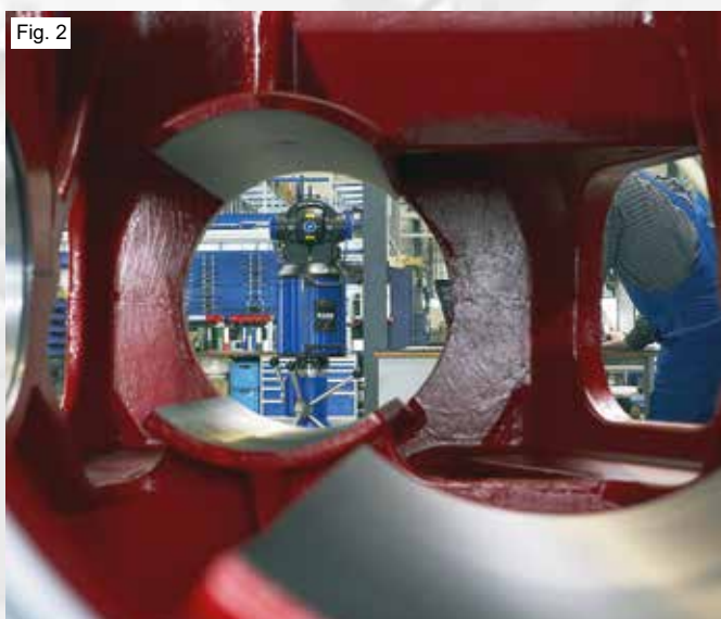
Fig. 1: Mechanical test run according API of 6-crank reciprocating compressor
