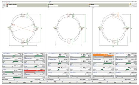
Thanks to the multi-strand capabilities of Profilemaster rebars can be measured in parallel on up to 4 strands:
