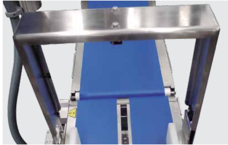
> Vertical detector on arch
