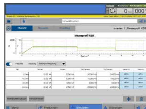
Welding profile with 4 sections and different frequencies
