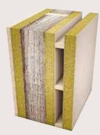
Perimeter wall with Strawpanel® cladding
