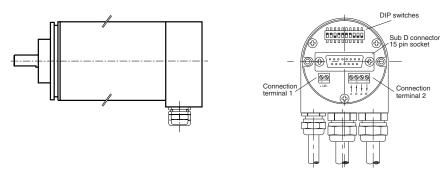
The connecting cap for triple connection technology is a T-coupler, which is installed in the PROFIBUS. It is equipped with three PG connections, which are subdivided as follows:
