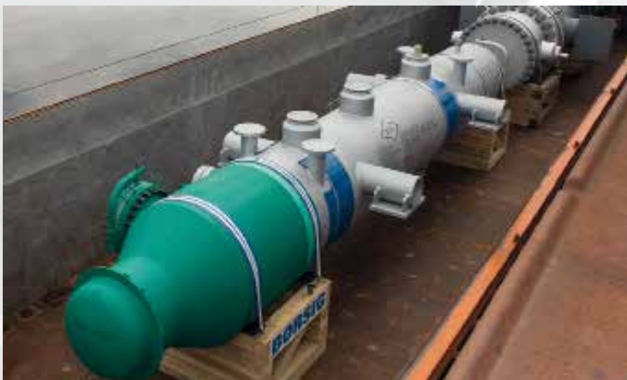
Waste heat boiler at the Borsig-Harbor
