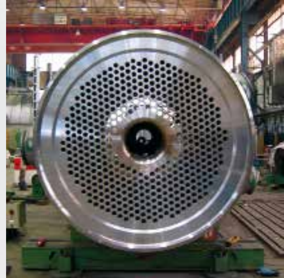
Gas inlet tubesheet with central bypass tube
