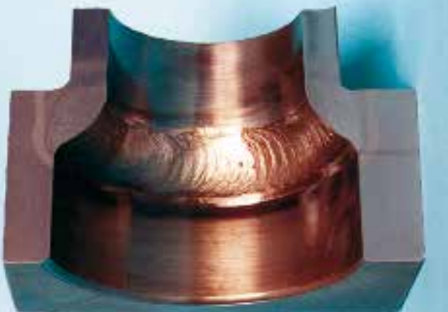
Specimen of tube to tubesheet weld
