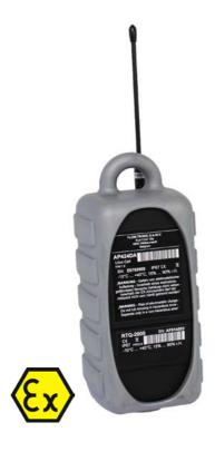
The RTQ-2000<sup>TM</sup> is a revolutionary device connecting directly to the Open Channel Non-Contact RAVEN-EYE® Radar Velocity flow sensor.
