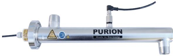
The UV-plant PURION 1000 H is made from electropolished stainless steel 1.4571. The PURION 1000 H is applied to disinfect drinking water up to a flow rate of 1.500 l/h and a transmission (or turbidity) of the water of at least 90% per cm.
