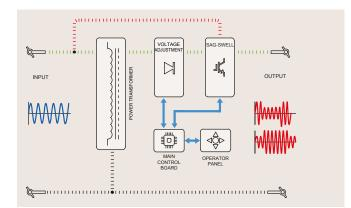
Test time in SSG simulator between 10msec.-999sec. and output voltages between 1% and 150% Vnom. can be adjusted. Voltage adjustment is made independently for each phase.
