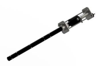
The AVI-MAG<sup>TM</sup> is a hot tap full profile electromagnetic averaging insertion flow meter. Multiple electrodes placed across the entire sensor body at **equal area**, measure and report the average flow rate over the full diameter of pipe. The specific design of the multi-electrode sensor compensates for variable flow profiles, including swirl and turbulent condition.
