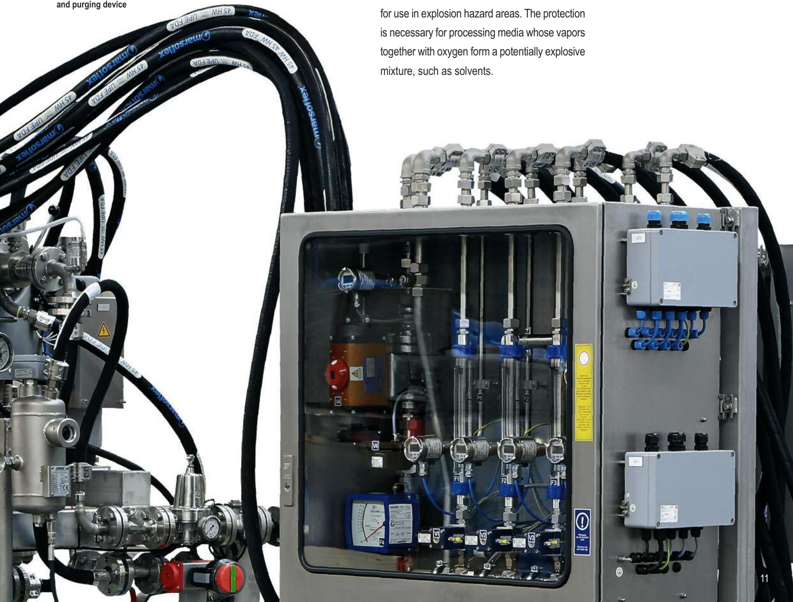
Mobile test unit with explosion protection and purging device
