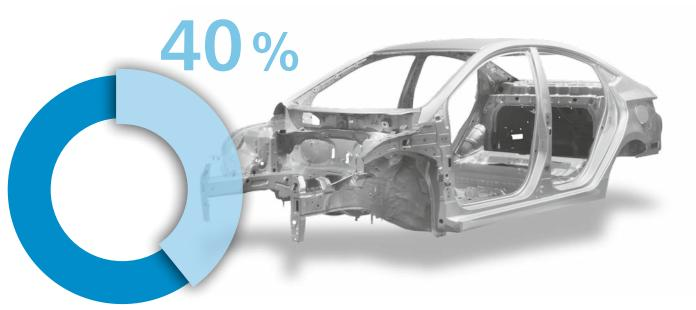
40% of a car's total weight is in the body. So it is a key element in moving car production towards more lightweight construction.
