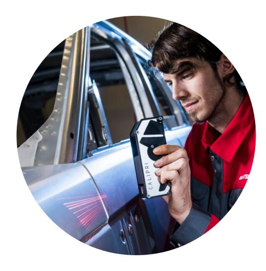
The optoelectrical profile measurement devices record the profile of edges and gaps without any contact. An intuitive swivelling movement offers evaluation of previously inaccessible profile forms without mathematical estimations. In addition, our patented tilt correction completely rules out user influences.
