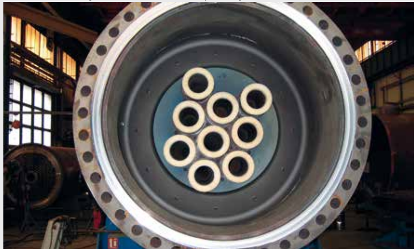
Inlet section with gas inlet nozzles of a BORSIG synthesis gas cooler
