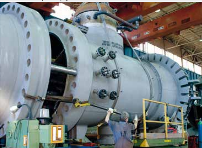
Lower vessel part of syngas effluent cooler (SHELL Gasification Process)
