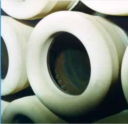
Ceramic coating of the gas inlet nozzles
