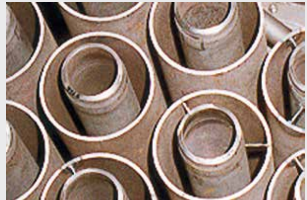
Assembly of connecting pipes and double tubes
