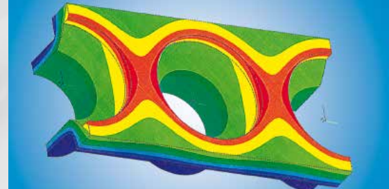
Fig. 26: Temperature distribution of tube inlet section by finite element analysis
