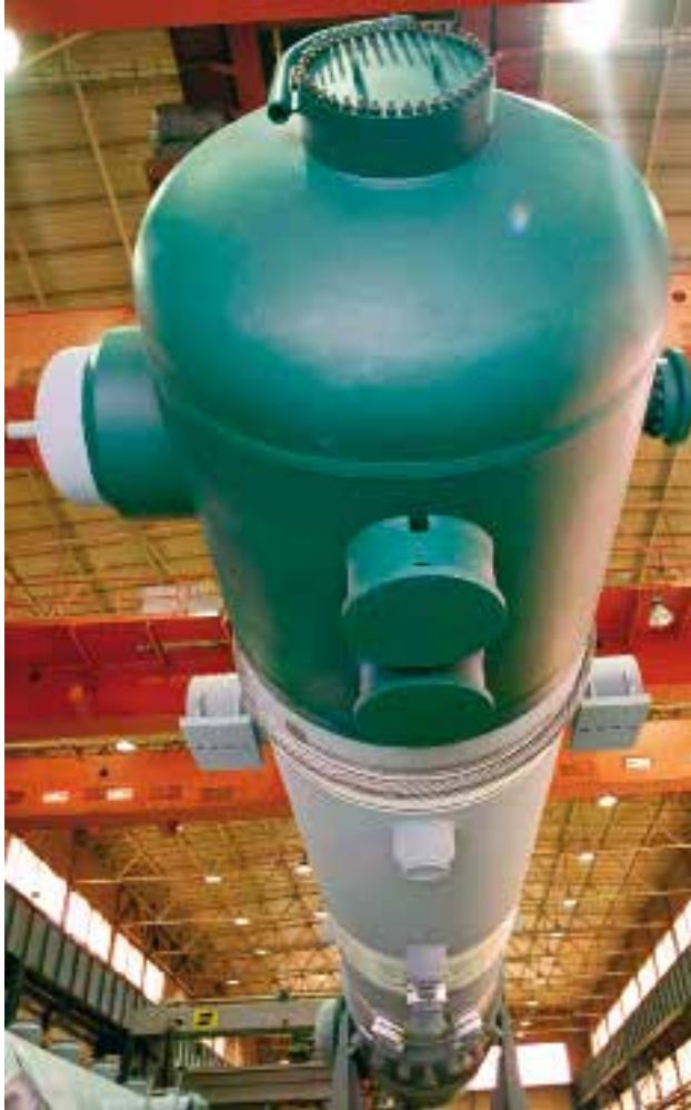
Process gas waste heat boiler
