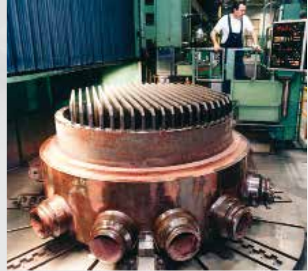
Machining of stiffened tubesheet system
