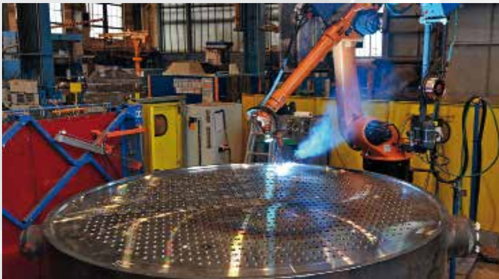
Automatic welding of stiffener fingers to tubesheet with robot
