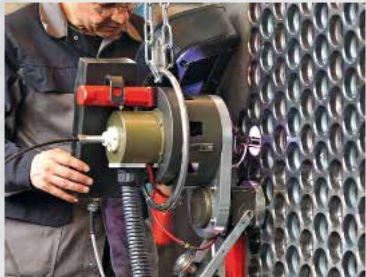
Automatic full penetration tube to tubesheet welding
