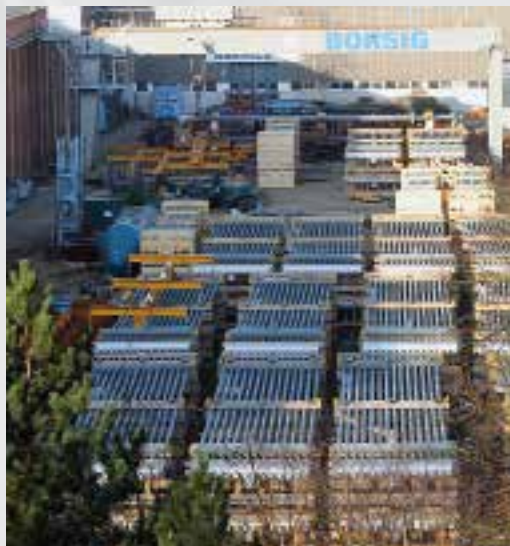
Linear transfer line exchangers
