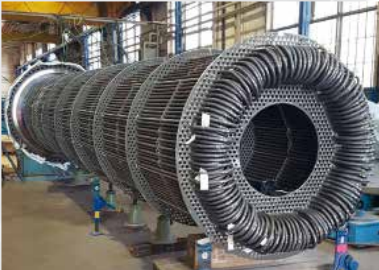
Works construction of a steam superheater
