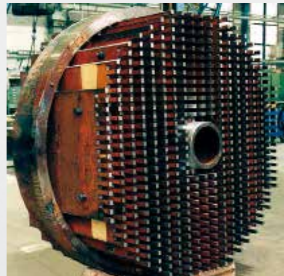
Presassembled stiffener system with integrated part of the bypass tube
