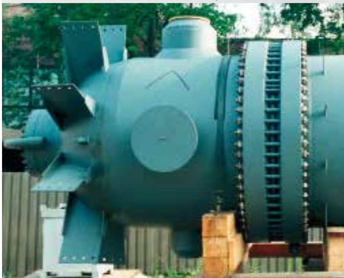
Combined steam inlet/outlet chamber of a steam superheater
