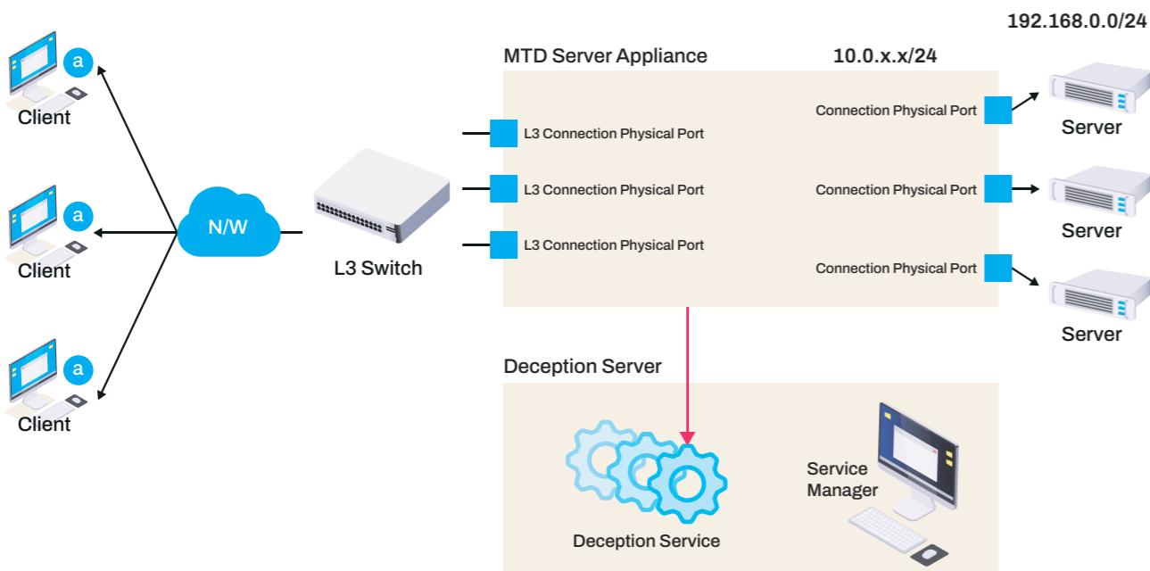
The Stealth MTD Server Appliance is a hardware appliance for protecting a server, which sends a response on behalf of the server when a client requests a service from the server.
