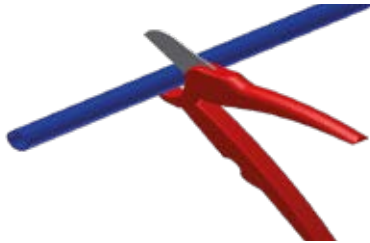
Step 1 Cut the PE pipe at right angle.
