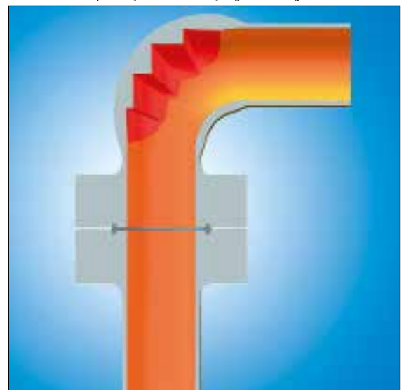
Connection of primary and secondary leg of twin leg BLQ
