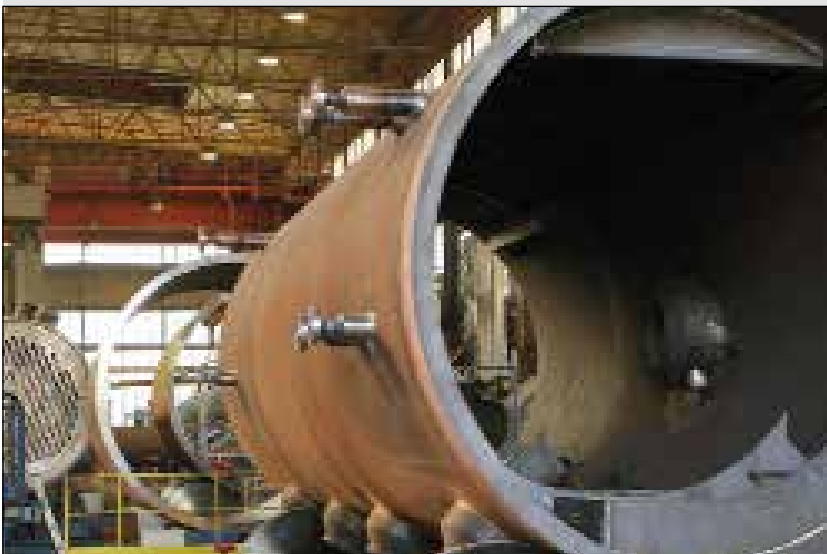
Manufacturing of steam drum
