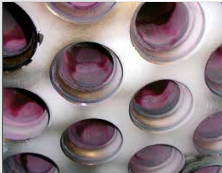
Penetration testing of TLE
