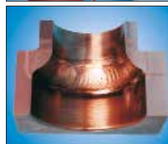
Specimen of tube to tubesheet weld
