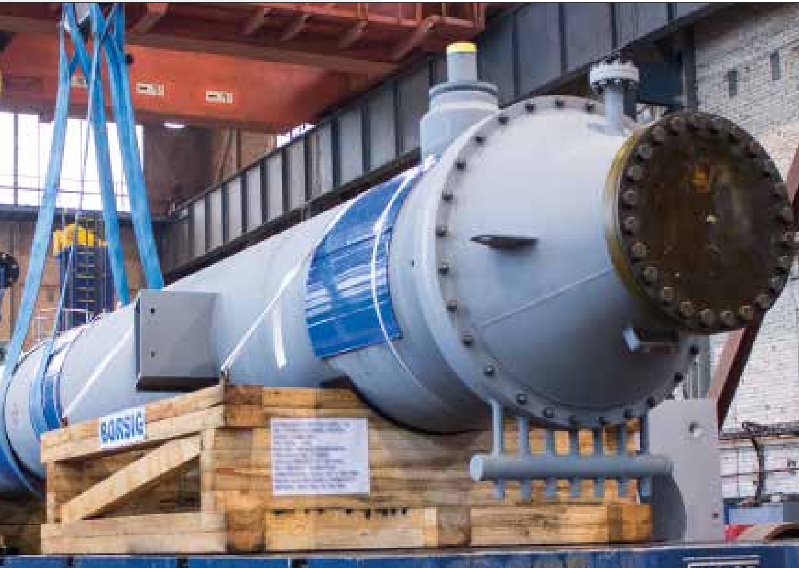
Transfer Line Exchangers at the works area
