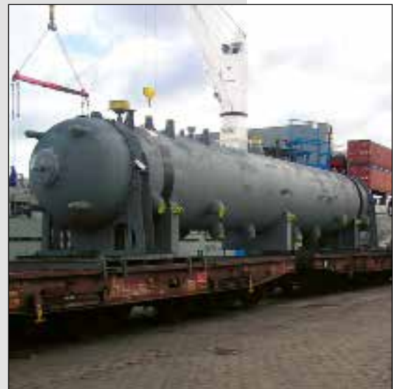
Steam drum ready for shipment
