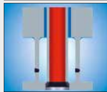
Fig. 10: Anchoring rib to gasinlet tubesheet weld
