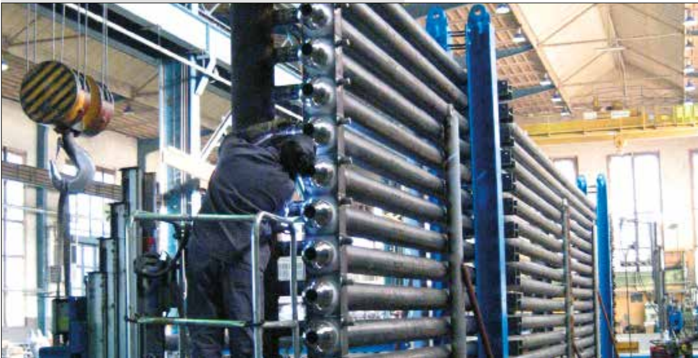
Manufacturing of "Linear" Transfer Line Exchangers
