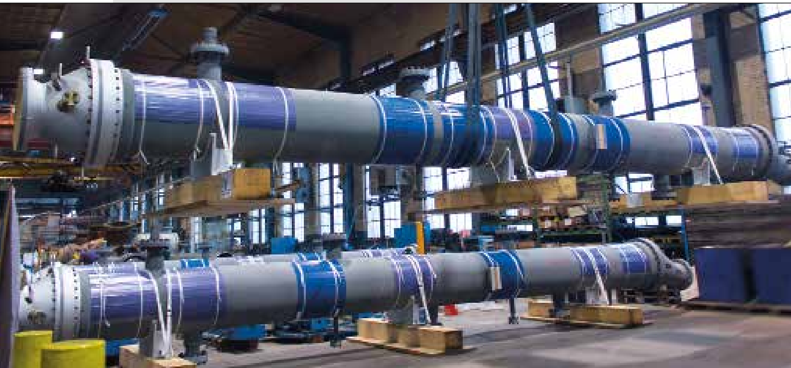
Manufacturing of "Tunnelflow" Transfer Line Exchangers
