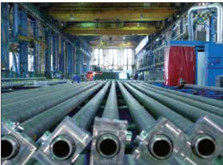
Double pipe elements in the workshop
