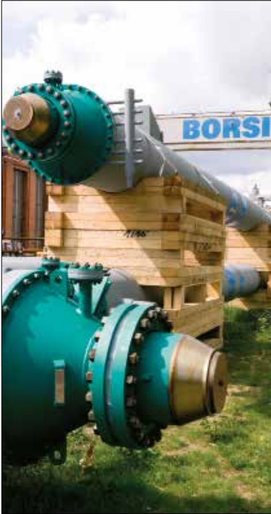
“Tunnelflow” TLEs ready for shipment
