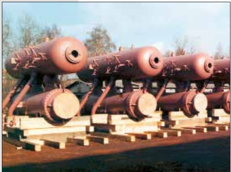
Compact Quench Systems ready for shipment
