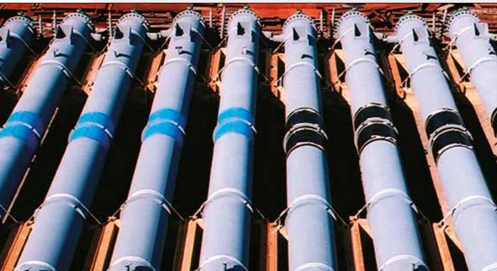
“Tunnelflow” Transfer Line Exchanger
