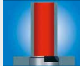
Fig. 9: Tube to tubesheet weld
