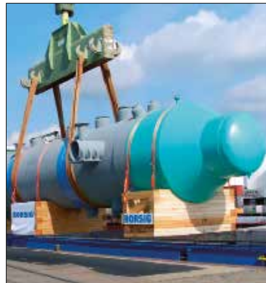
Process gas waste heat boiler
