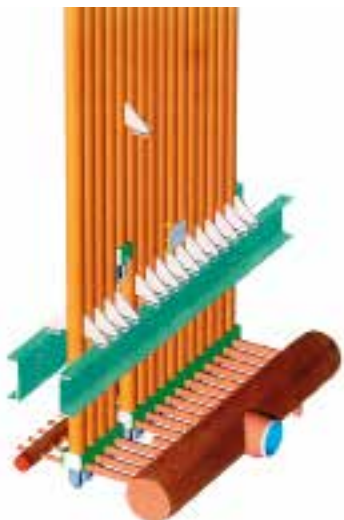
Cutting process / waterside connections lifting upwards
