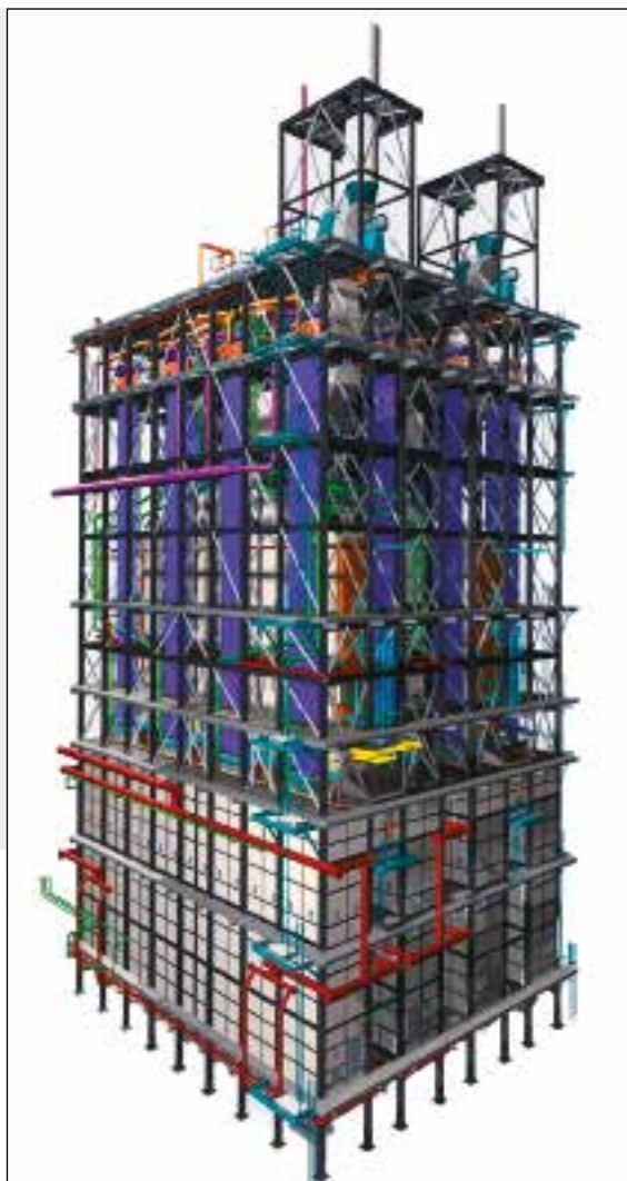
Computer simulation of two naphtha cracking furnaces
