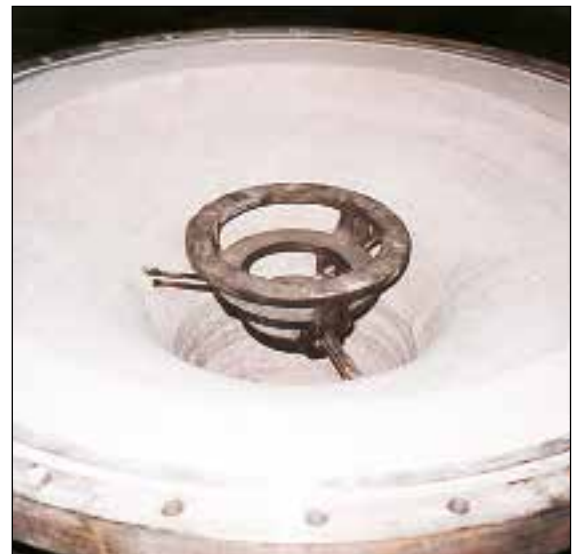
Erosion protection shield
