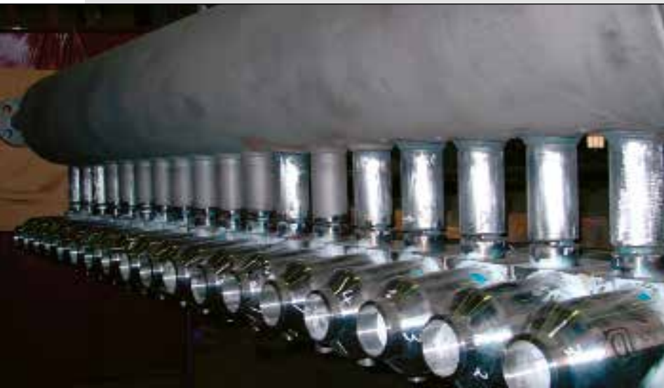
Gas inlet heads with BfW supply header
