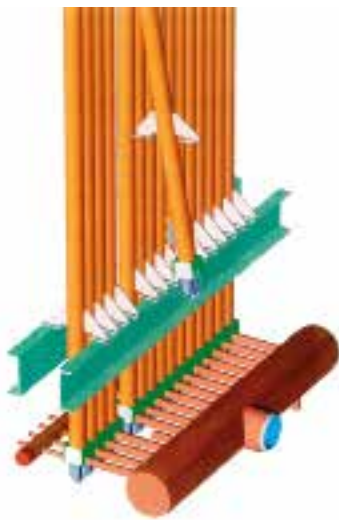
Removing of BLQ double pipe out of the module
